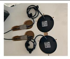
1. Unplug front or rear hand control frm the coupler directly below the front of the worksurface for 30 seconds for all power to drain from the hand control.
