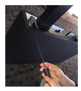
4. If still not working, use the Allen wrench tool that came with your Xybix product manual to get into the black lift case that is closest to the CPU cabinet.
