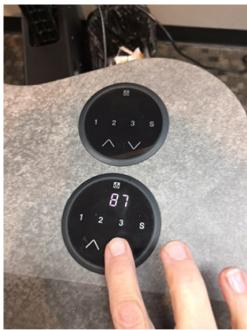
2. Plug hand control back in and wait 30 seconds for the power to come back into the hand control. Next, make sure anything under the work surface is cleared away (i.e. trash cans, equipment) and hold the down button. Keep holding until it reaches the lowest position and bounces up slightly. If table starts going crooked, stop immediately, and call Xybix Customer Service at 720-382-2114 or 720-382-2122. If table resets fully, you should be able to adjust your table to the appropriate height.
