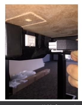
3. If this does not solve the problem, check that leg extension cables are plugged in fully into the leg ports at the top of the less underneath the the laminate surfaces. Try resest again.
