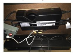
**Step 1** - Locate the control box under the front or rear work surface that is having the issue.
