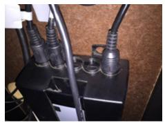
**Step 3** - Swap the cables for the two legs with each other. The leg cables are the ones that are next to each other (the cable on its own is the hand control cable).
