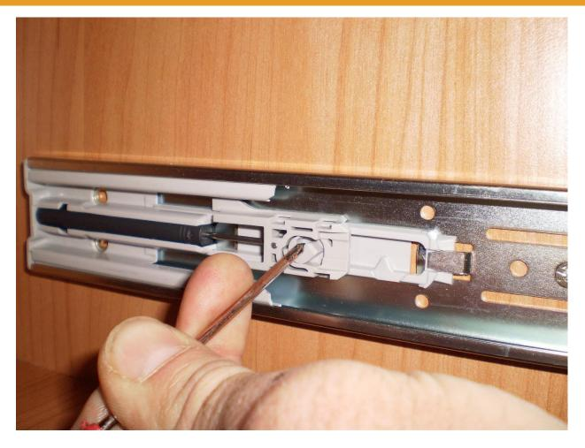
Using a flat head or Philips head screwdriver turn the release lever Counter-Clockwise (to the left) as shown.
