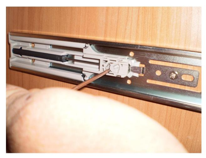
To re-place the release lever back again pull the mechanism all the way forward until it locks into place as shown.
